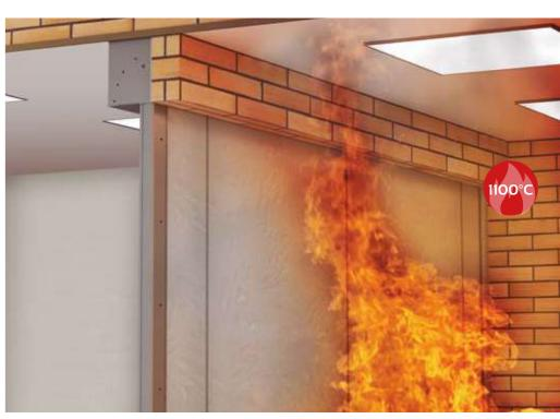
Fire curtain tested with the supporting elements (headbox and side guides) exposed directly to fire.
